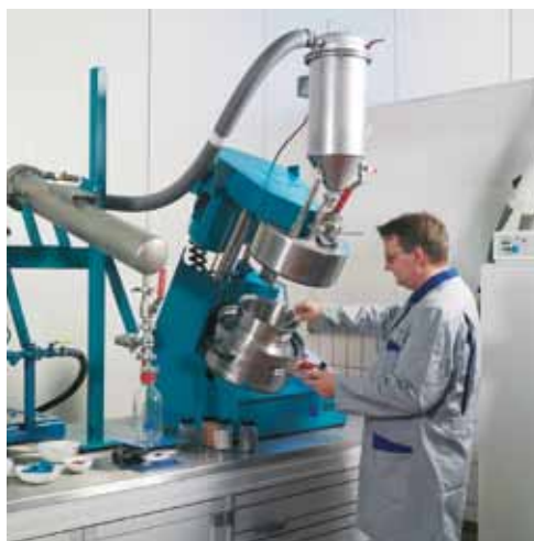
Laboratory mixer for applications under vacuum on the basis of the EVACTHERM® principle for product development or small-scale production
