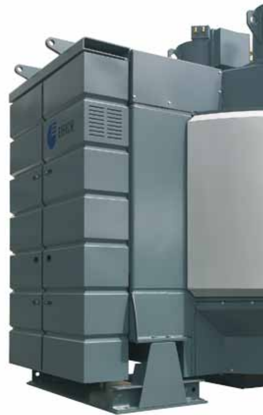
Mixer with a usable volume of 12,000 liters for the preparation of iron ores and sinter mixes
