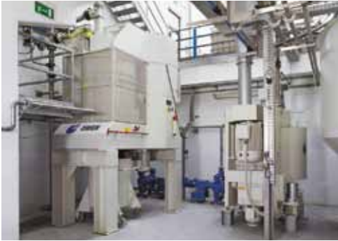
A combination of a MaxxMill® and intensive blunger for the preparation of ceramic slurry for the production of large tiles
