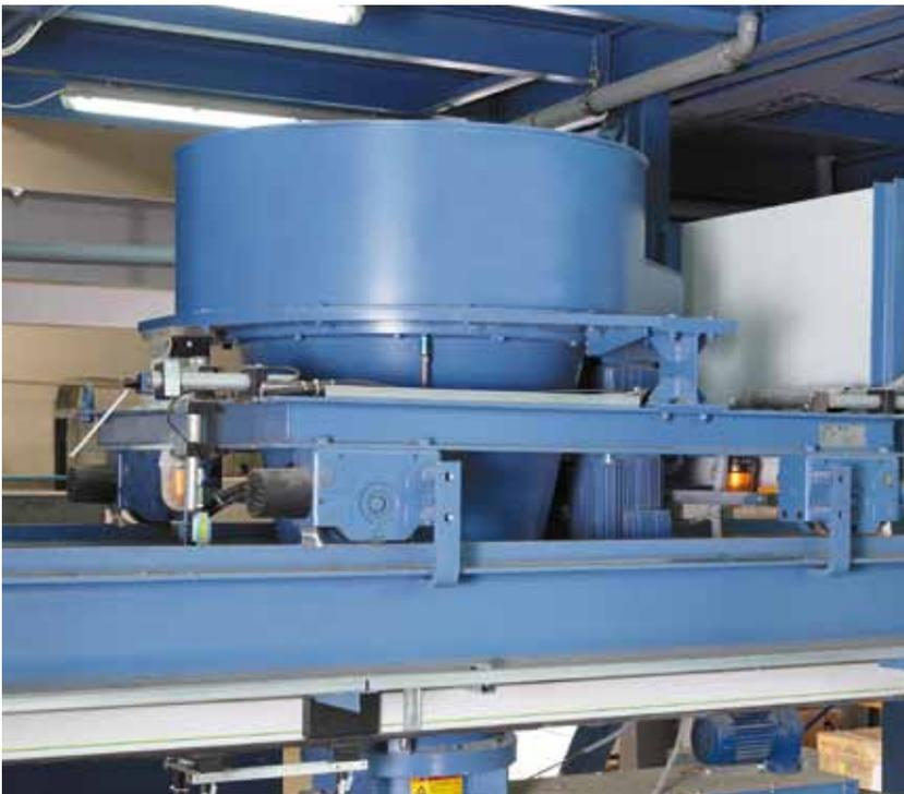
The paste feeders are mobile and ensure a continuous supply of material to the pasting lines. One paste feeder is used for each pasting line. Several pasting lines can thus be supplied by one EVACTHERM® system.
