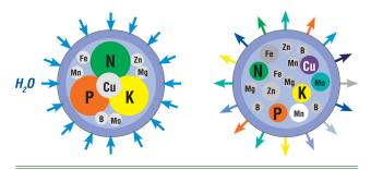
**Figure 1.** Nutrient release. Left: every fertilizer granule contains all the nutrients; the nutrients are dissolved by water. Right: a concentrated nutrient solution is created; the nutrients are released in a controlled manner.
