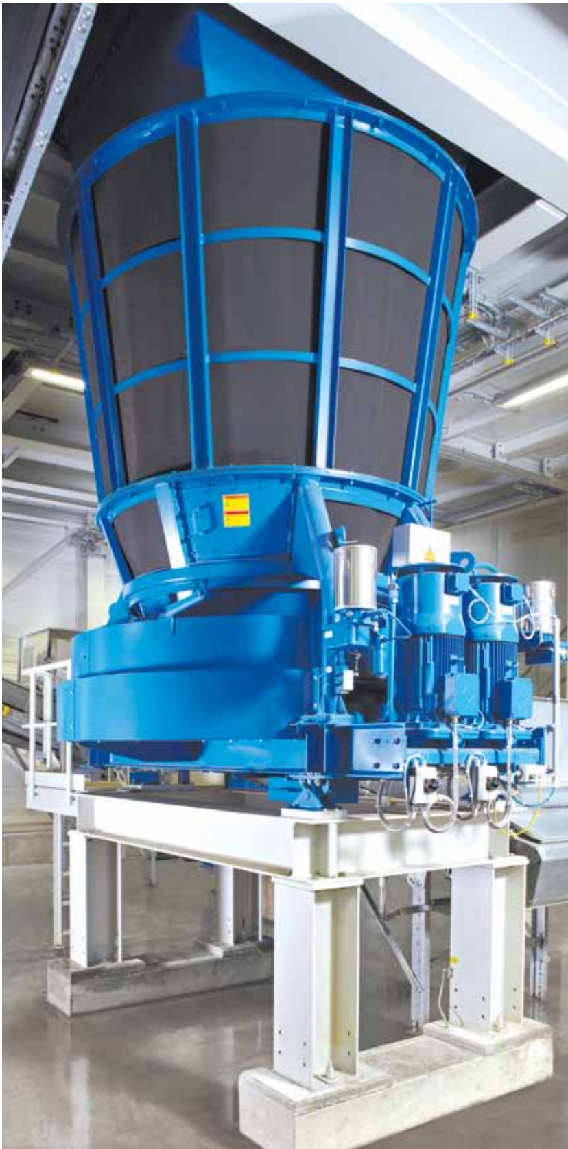
Picture 1 UE25 table feeder in a foundry with a material feed hopper for a volume of 9000 liters
