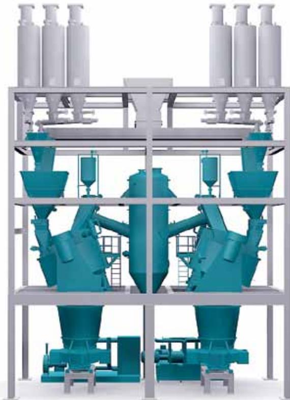
Fig. 6.2: Partial system layout with a throughput of roughly 260 t/h (286.6 short tons/h) of finished sand. It shows two EVACTHERM® RV32VAC mixer-coolers (7 m³ = 247 ft³ per batch) for multiple molding lines with shared peripheral cooling equipment.
