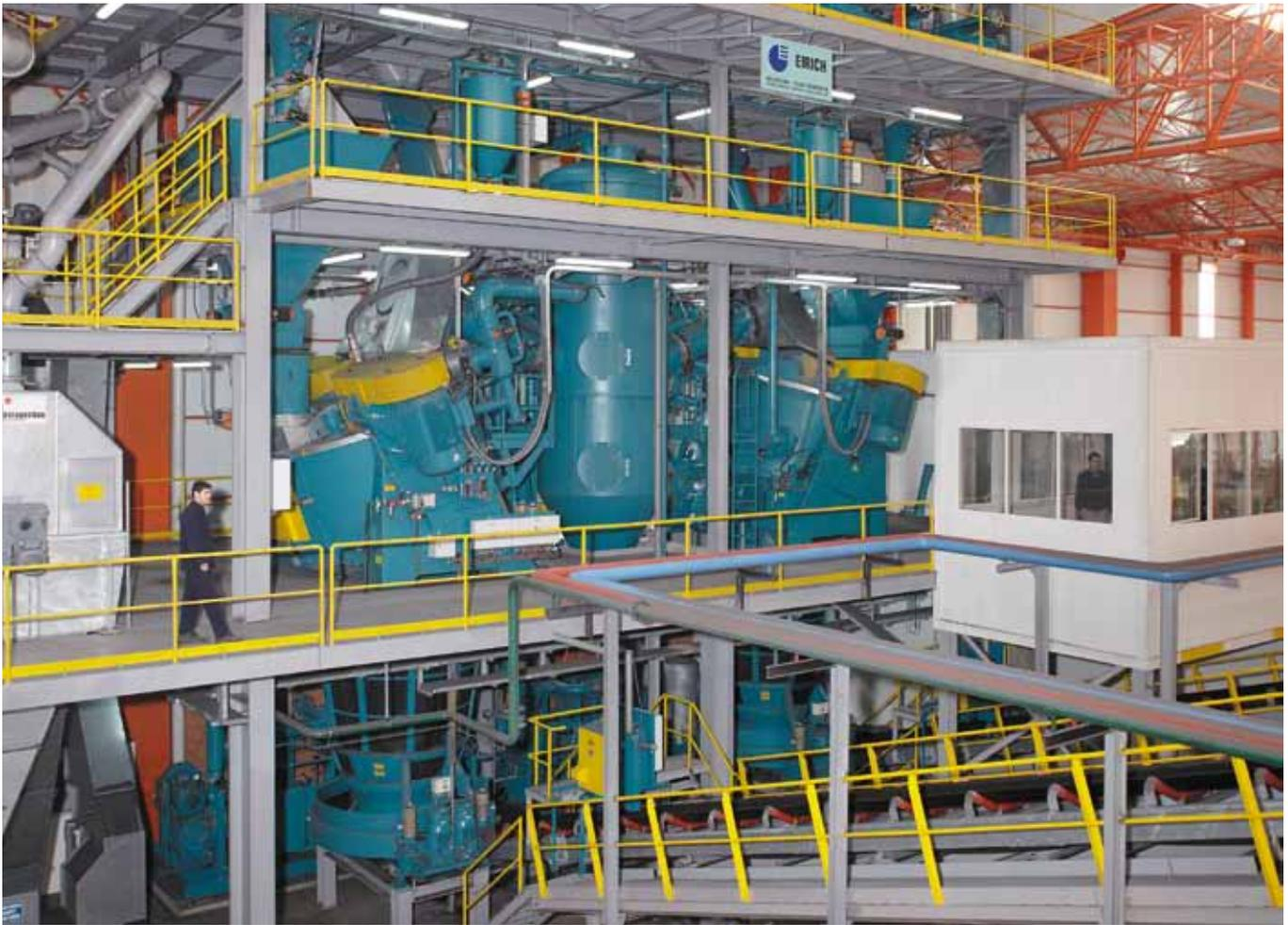
Fig. 6.1: Two EVACTHERM® RV32VAC mixer-coolers (7 m³ = 247 ft³ per batch) for roughly 260 t/h (286.6 short tons/h) production demand.
