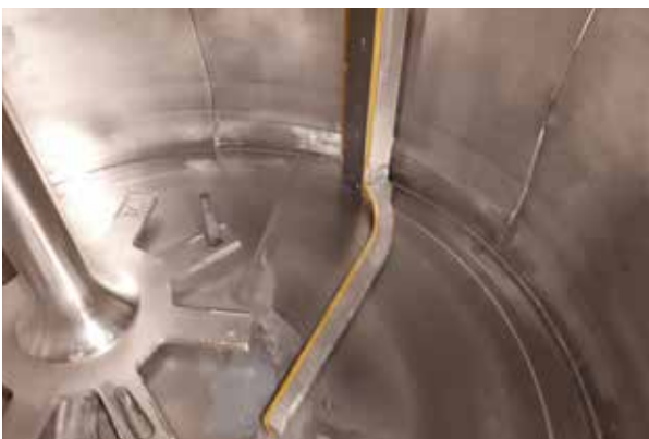
Interior of the mixing pan with mixing tool and touching bottom/wall scraper
