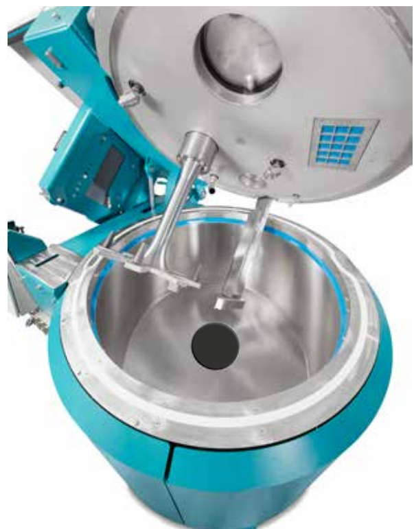
Mixing pan with no joints or gaps
